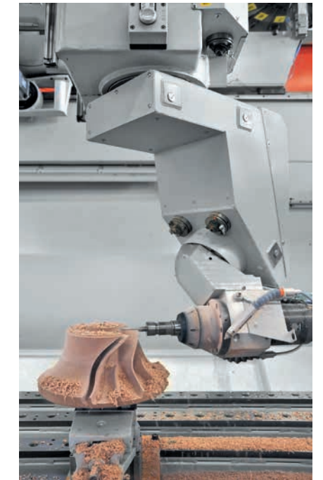
Machining of an impeller from ureol (Cibatoool) by the cardanic 5-axis working head of an ECO-NT.
