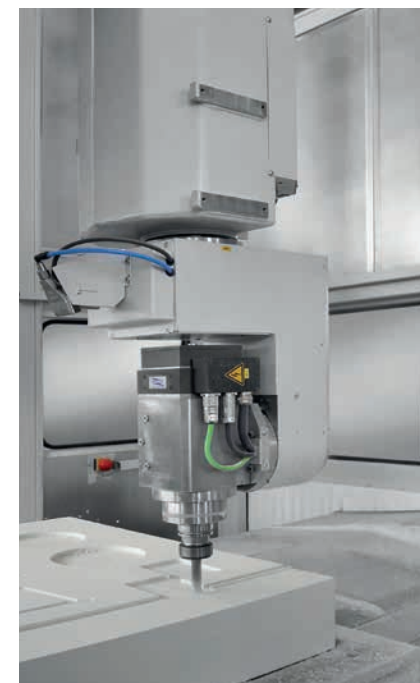
Machining of PU-foam in the ECO-2616 A, 5-axis fork-shaped working head, Z-stroke 1,300 mm.
