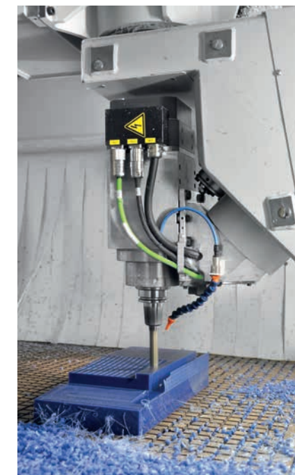
Chip removal at a finished plastic component (wedge) for beverage bottling in the VISION-I-H, cardanic 5-axis working head, Z-stroke 780 mm.
