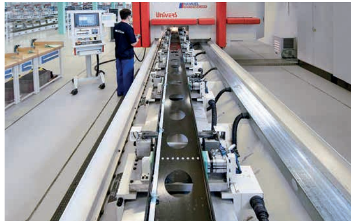
Machining centre UNIVERS with an H-profile carrier for aircraft floor construction clamped in the machine.
