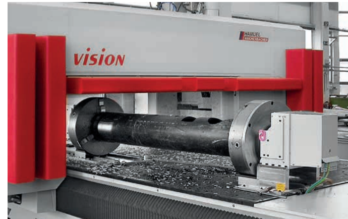
Pipeline machining on an additional NC-lathe (up to \varnothing 600 mm).
