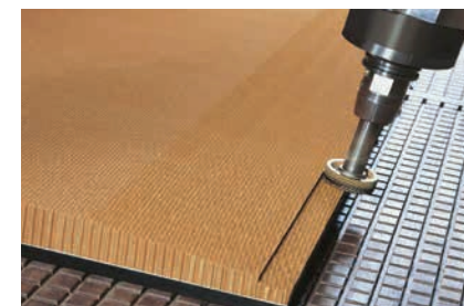
Machining of a honeycomb core, e.g. for reinforcing aircraft wings.
