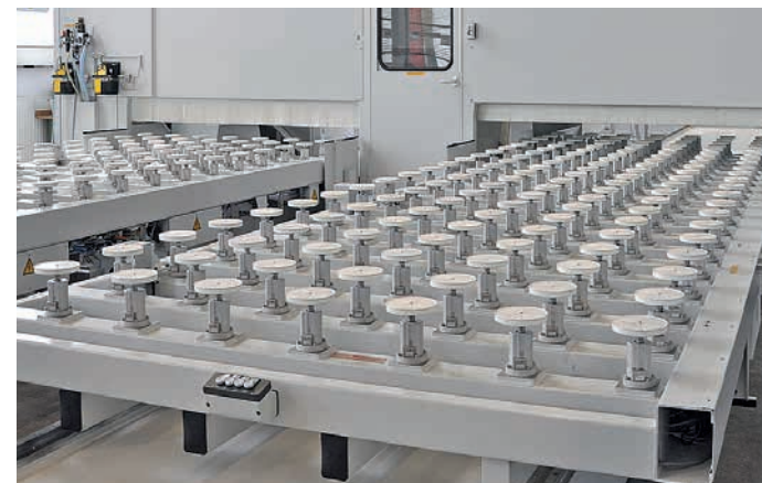
Machine tables of an ECO with 147 pins, each, for caravan walls.
