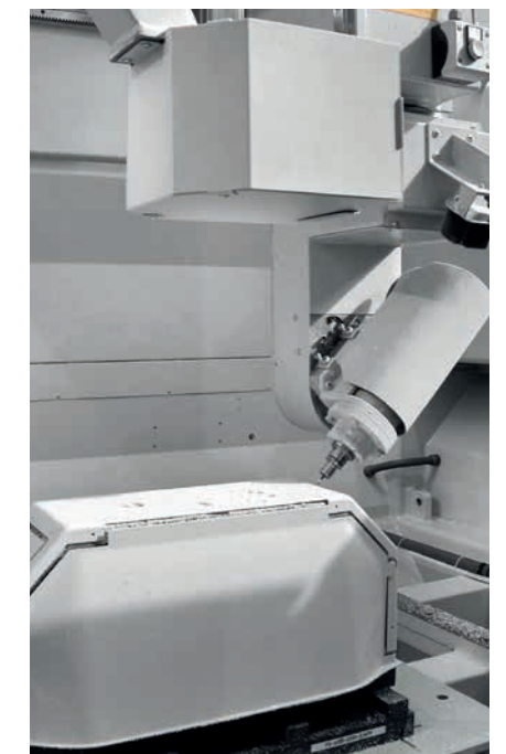
Milling of a preformed plastic component in the ECO-NT, 5-axis fork-shaped working head, Z-stroke 1,000 mm.
