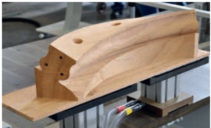
Interpolating 5-axis machining. The handrail is completely machined and cut to length. Design and programme established by your software company.
