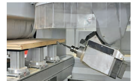
Cardanic 5-axis working unit (spindle 24 kW, undercut 20°) for the machining of solid wood.
