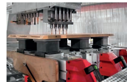
Machining of a furniture body part with a 15-spindle drilling unit in an ARTIS.
