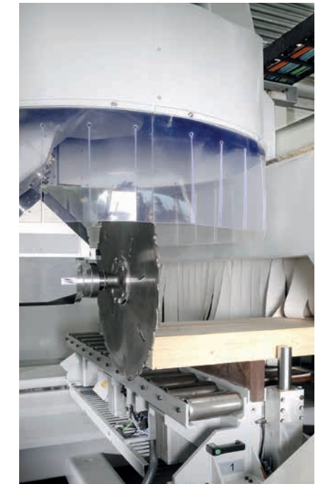
Glulam-machining (up to 50 m) with a 5-axis working unit (spindle 55 kW, saw blade 800 mm).
