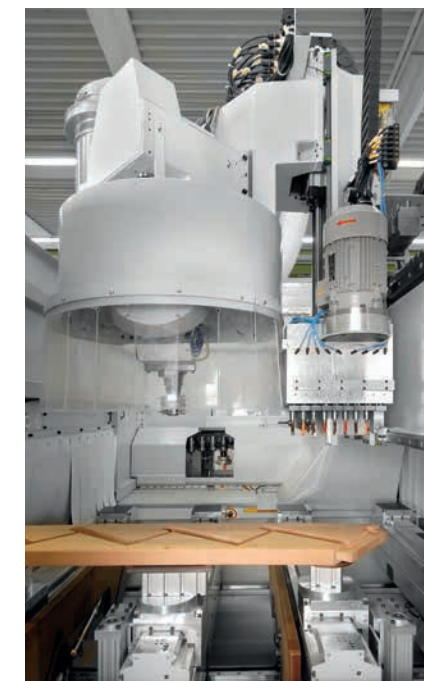
Automatic beam table, multi-spindle drilling unit with 25 places and chain tool magazine with 36 places.
