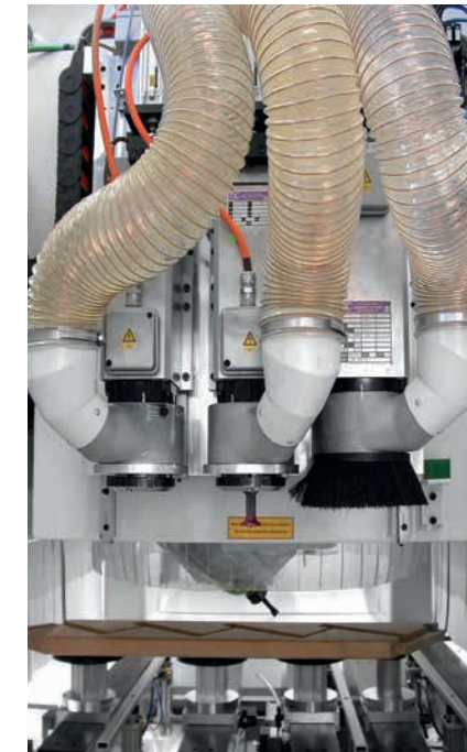
Working units of a VISION-ST (staircase production) with 5 axes and three additional milling motors.
