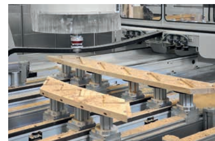
Machining of staircase strings on an ECO with 2 automatic beam tables.
