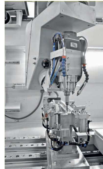
Cardanic 5-axis working unit for the efficient 6-side complete machining of formed parts and profiles.
