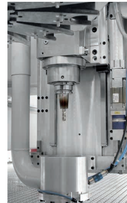
VISION with NC-height adjustable extraction bell to account for the different lengths of the milling tools during machining. The spindle is equipped with a rotary feed-through for coolant.
