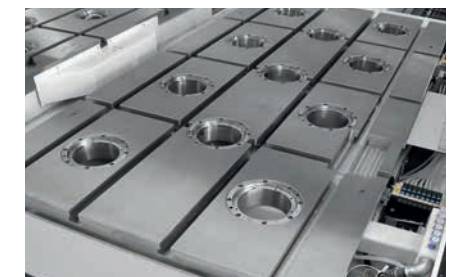
Coordinate table of an ECO – a special design for the high demands of the aircraft industry.
