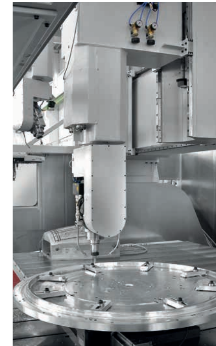
Machining of an aluminium ring for an aircraft engine in the ECO-machining centre with T-groove tables.
