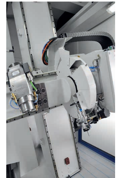
5-axis working unit of an ECO-RS with a tool changer with 12 places at the C-axis. Another tool changer with 6 places is installed in a lateral position at the machine bed.
