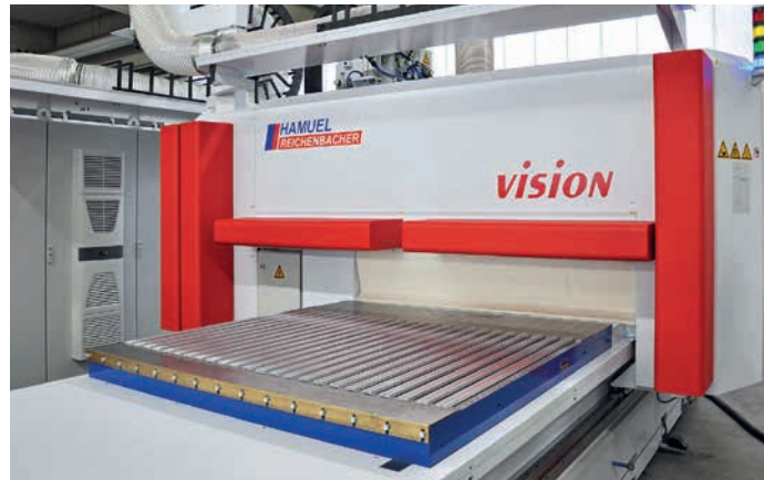
Stationary machine table with steel base frame equipped with two magnetic clamping plates.
