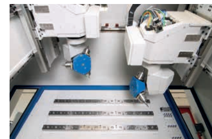
Cardanic star-shaped milling heads (optional version) for the ECO-RS with inclined machine bed.
